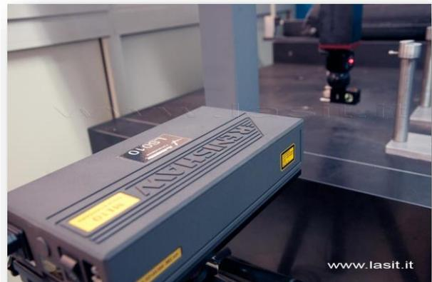
To satisfy the most stringent requirements, Laser Americas can provide a specific machine calibration with a test certificate. The positioning straightness of the motion of each single axis is measured with an interferometer. The positioning data is taken with an interval of 20 or 50 mm and the results are stored in the calibration table of the software. According to this table software commands the motors in order to compensate for mechanical errors.
